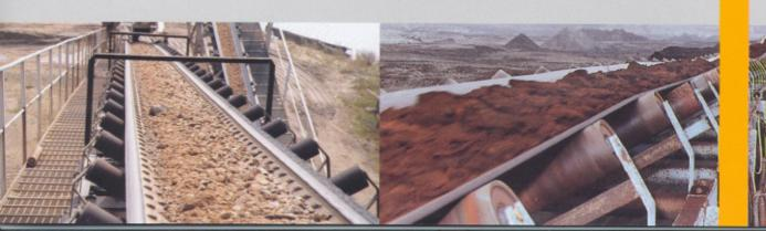
CONTIFLEX® textile conveyor belts fulfil a wide variety of transport tasks in all types of industry. In addition to a range of belts for normal bulk goods, various special types are available for conveying hot goods, for the transport of goods containing oil and grease, for steep-incline conveying and with special reinforcing materials for particular applications.
